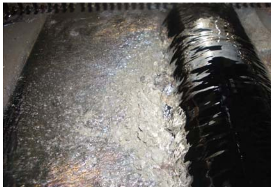
Lead-free solder bath without MS2™ molten solder surfactant, showing typical dross buildup
