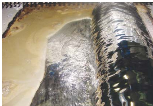
Lead-free solder bath with MS2™ molten solder surfactant, showing no dross—only shiny solder
