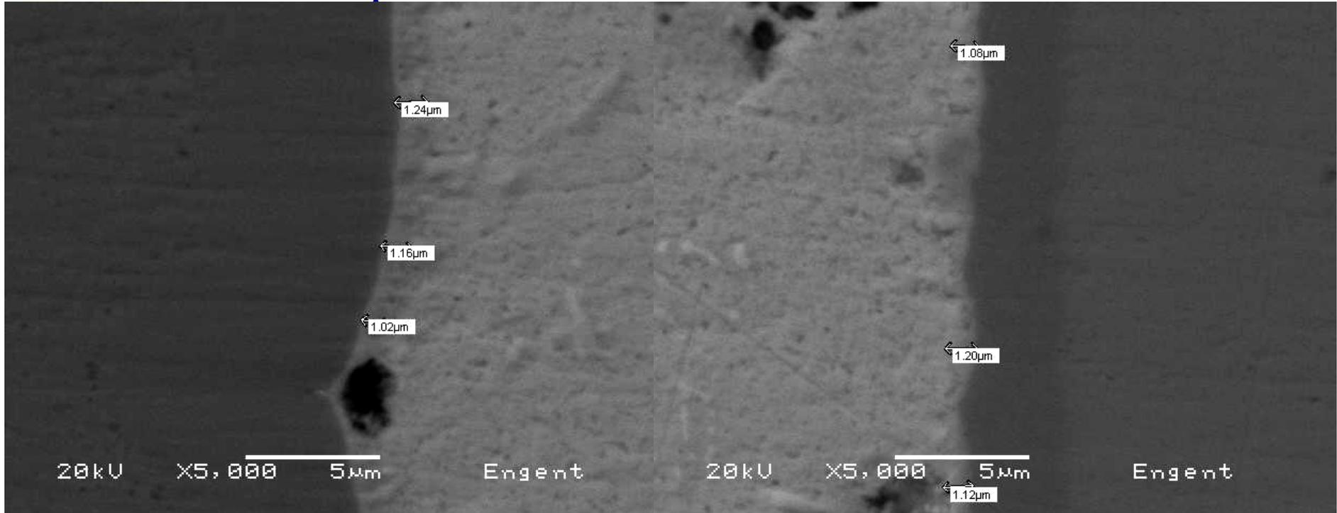
Board 4 showing overall image of DIP Pin and solder grain structure
